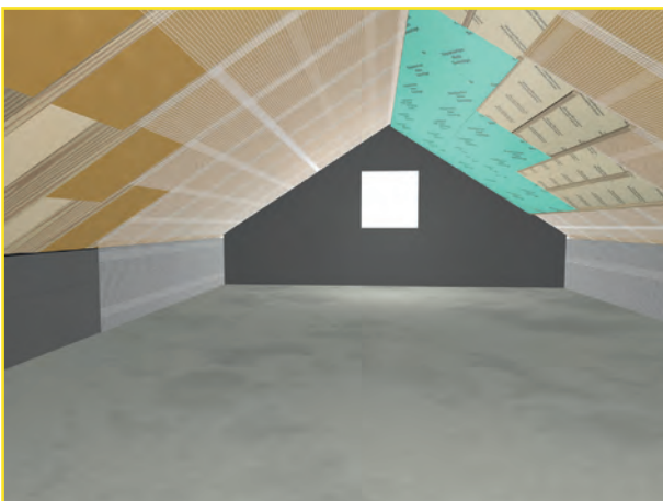
Fig. 16: Laying on rafters or between two layers of panels. Earthing diagram see Fig. 16a
