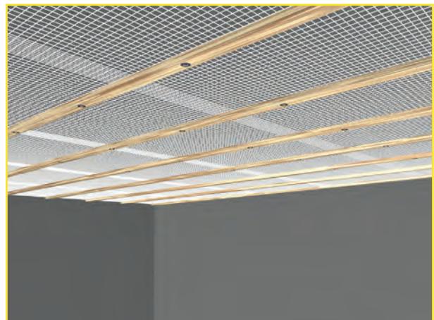
Fig. 5: Fixed fastening of the sheets with the help of the battening - Removal of the auxiliary nails
