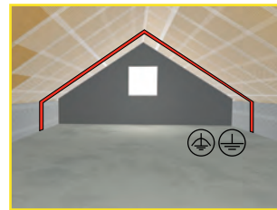
Fig.25a: Grounding roof slope with EEB
