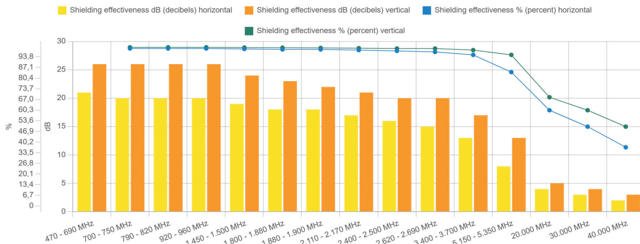
Shielding effectiveness - Antiwave OC black - stretched - 470 MHz to 40.000 MHz (40 GHz)
