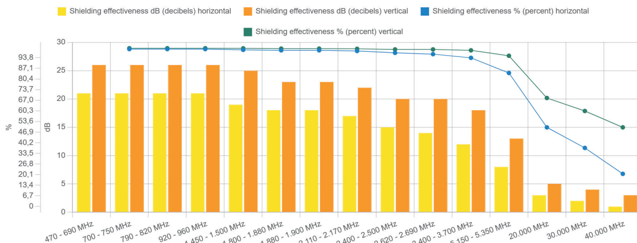
Shielding effectiveness - Antiwave OC white - stretched - 470 MHz to 40.000 MHz (40 GHz)
